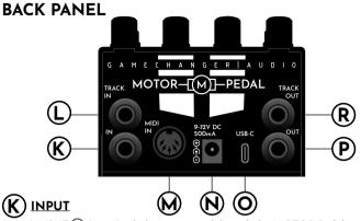
MAIN INPUT (K) (mono), which passes signal through the MOTOR Pedal to the MAIN OUTPUT (F); it's VOLUME is adjustable with the CLEAN VOL knob (F)
