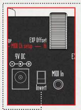
When the switch is **DOWN**, the pedal will behave as expected the long end of the foot-pedal will produce a pitch-down effect and the curved end will pitch the signal upwards.
